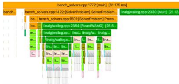
Figure 21: The last part is the top preconditioned conjugate gradient. Everything is now generated, embedded and fused in a whole big kernel. For this benchmark and these options, we are going from 95ms down to 22ms, which represents a reduction by a factor of more than four.
